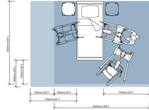
Blue area shows the minimum working area required to enable the caregiver to use the floor lifter ergonomically from one side.
